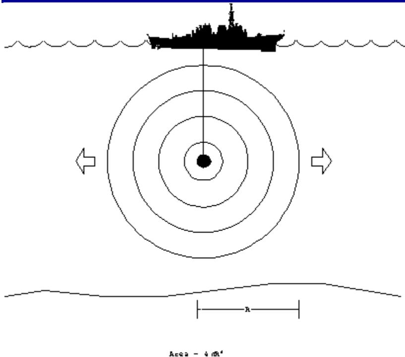
The equation for the decrease in signal energy of the sound as it spreads out to range R, the Transmission Loss (TL), is:
