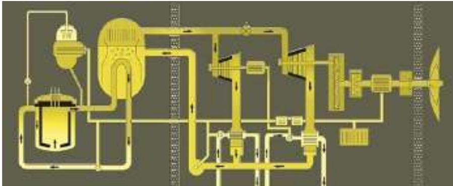
Figure 1: Pressurized water nuclear propulsion plant
