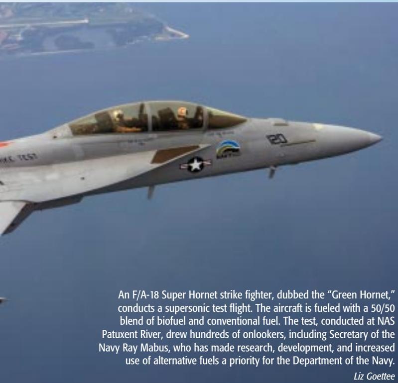
An F/A-18 Super Hornet strike fighter, dubbed the “Green Hornet,” conducts a supersonic test flight. The aircraft is fueled with a 50/50 blend of biofuel and conventional fuel. The test, conducted at NAS Patuxent River, drew hundreds of onlookers, including Secretary of the Navy Ray Mabus, who has made research, development, and increased use of alternative fuels a priority for the Department of the Navy.
